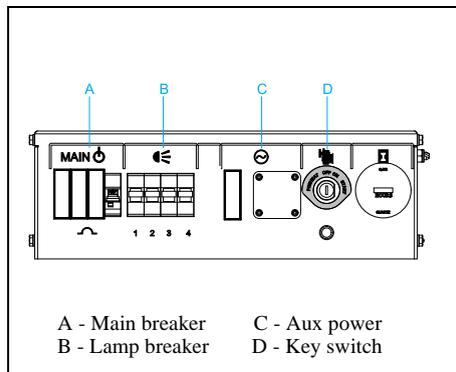
**Figure 3.8 Circuit breakers/power switch**
