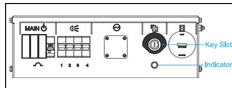
**Figure 3.7 Key slot and glow-plug indicator on main control panel**
